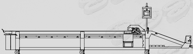
Polyline PMML 102 (6.2 m) with inclined infeed section and belt flour dusting system
