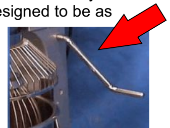
Picture 3. The handle and bowl of the machine must be raised to engage the electrics of the mixer.
